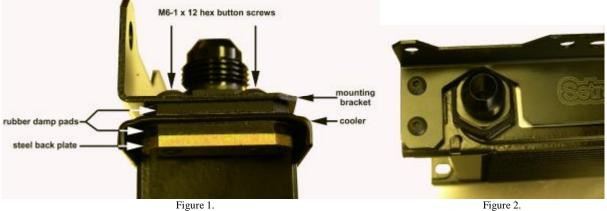
2. Place steel back plates, rubber damping pads toward mounting bracket, under each tab and use included screws to attach.
